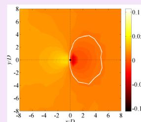
(right) contour plot of coefficient of pressure (left) contour plot of difference of pressure of a single WT at  $h/D=2.5$
