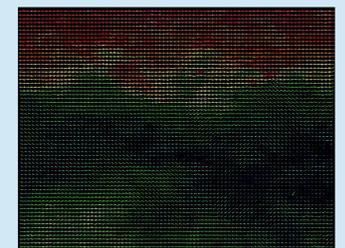
PIV image in far-wake region of a single WT with a overlap of 50%. Wind direction is from right to left
