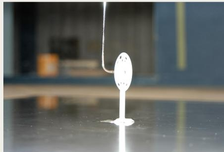
Single wind turbine model located at the geometric center of the pressure plate
