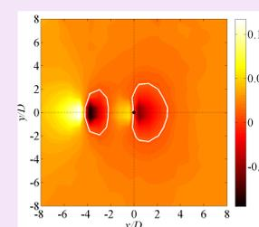
(right) contour plot of coefficient of pressure (left) contour plot of difference of pressure of two WTs with an interval of  $x/D=4.0$
