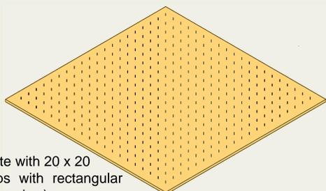
Pressure plate with 20 x 20 pressure taps with rectangular shape (bottom-view)
