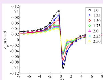
Centreline pressure variation with hub height provides a quantitative comparison and clearly indicates that the pressure footprint decreases in terms of  $c_p$  as the hub height increases
