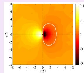
(right) contour plot of coefficient of pressure (left) contour plot of difference of pressure of a single WT at  $h/D=1.0$
