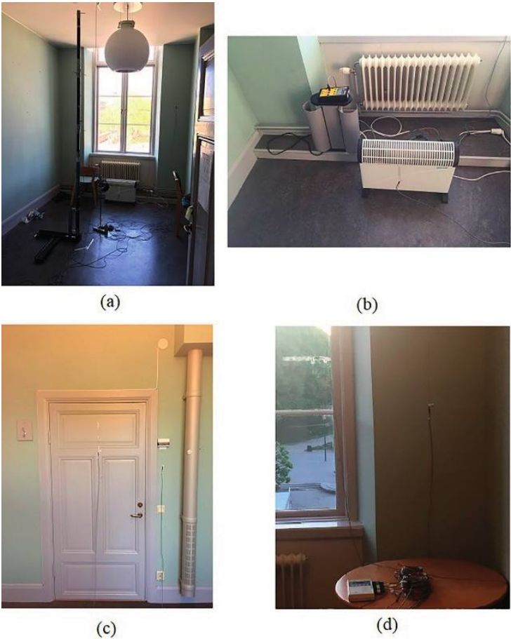
Figure 3. (a) The vertical rod for the office room’s air temperature measurement, (b) The electrical radiator connected to the energy logger, (c) Temperature thermistor sensors attached to the surfaces of internal wall and door, and (d) Temperature thermistor sensors attached to the inner surface of the external wall and window.
